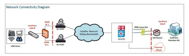
As per above diagram, the left part depicts the remote VSAT & LAN setup diagram, the middle part about the satellite bandwidth and Hub and the right part about SunPetro HQ/Internet. Provider has to install one Ku and one XC VSAT (Fixed 1.8m antenna) with RJ-45 Ethernet drop from Ku & XC indoor modems (Remote CPE). Both the links will be directly terminated to SunPetro Fortinet firewall (FW) WAN ports at RIG.
